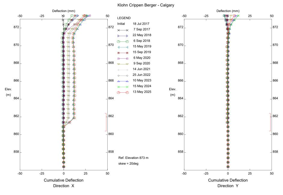
C060; H597:02, Slide East of Blackfalds, Inclinometer SI17-C60-02
