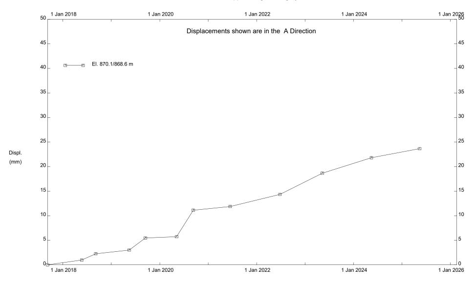
C060; H597:02, Slide East of Blackfalds, Inclinometer SI17-C60-01
