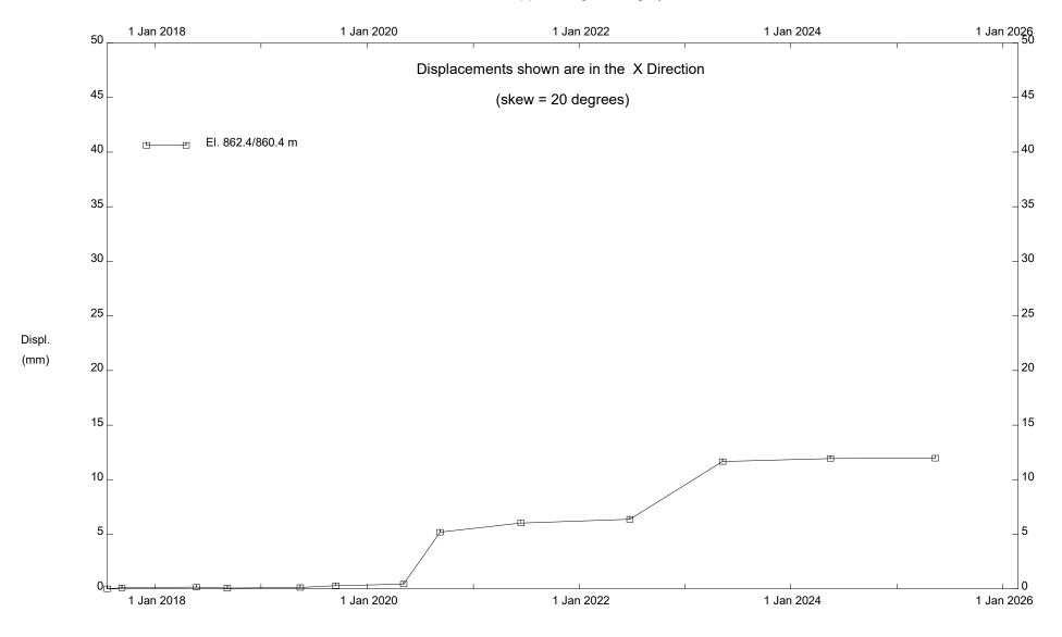
C060; H597:02, Slide East of Blackfalds, Inclinometer SI17-C60-02
