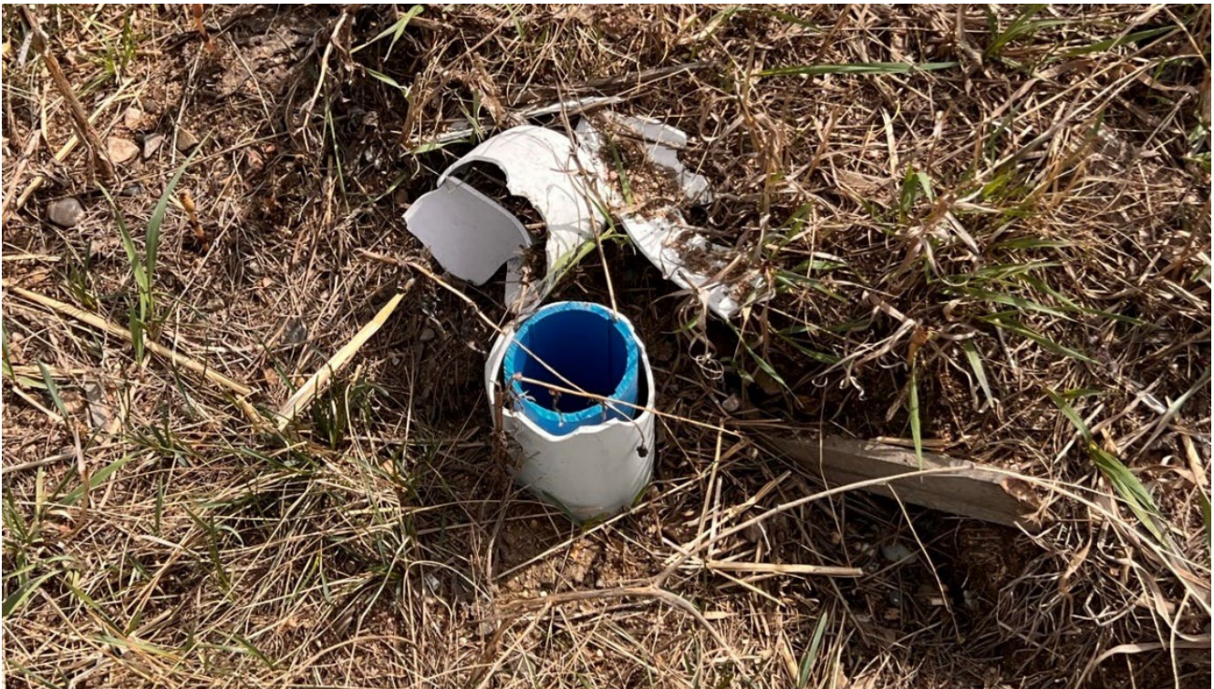
Photo 1 Damaged PVC casing protector at SI21-C43-01. Photo taken May 8, 2023.
