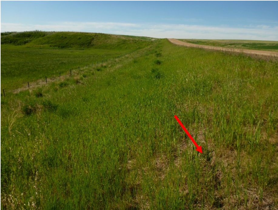
Photo 2 Photo showing evidence of ground cracking extending to the north as indicated by the red circle (waypoint 703) of the backscarp (1-2m) Photo taken June 13, 2018 looking north.
