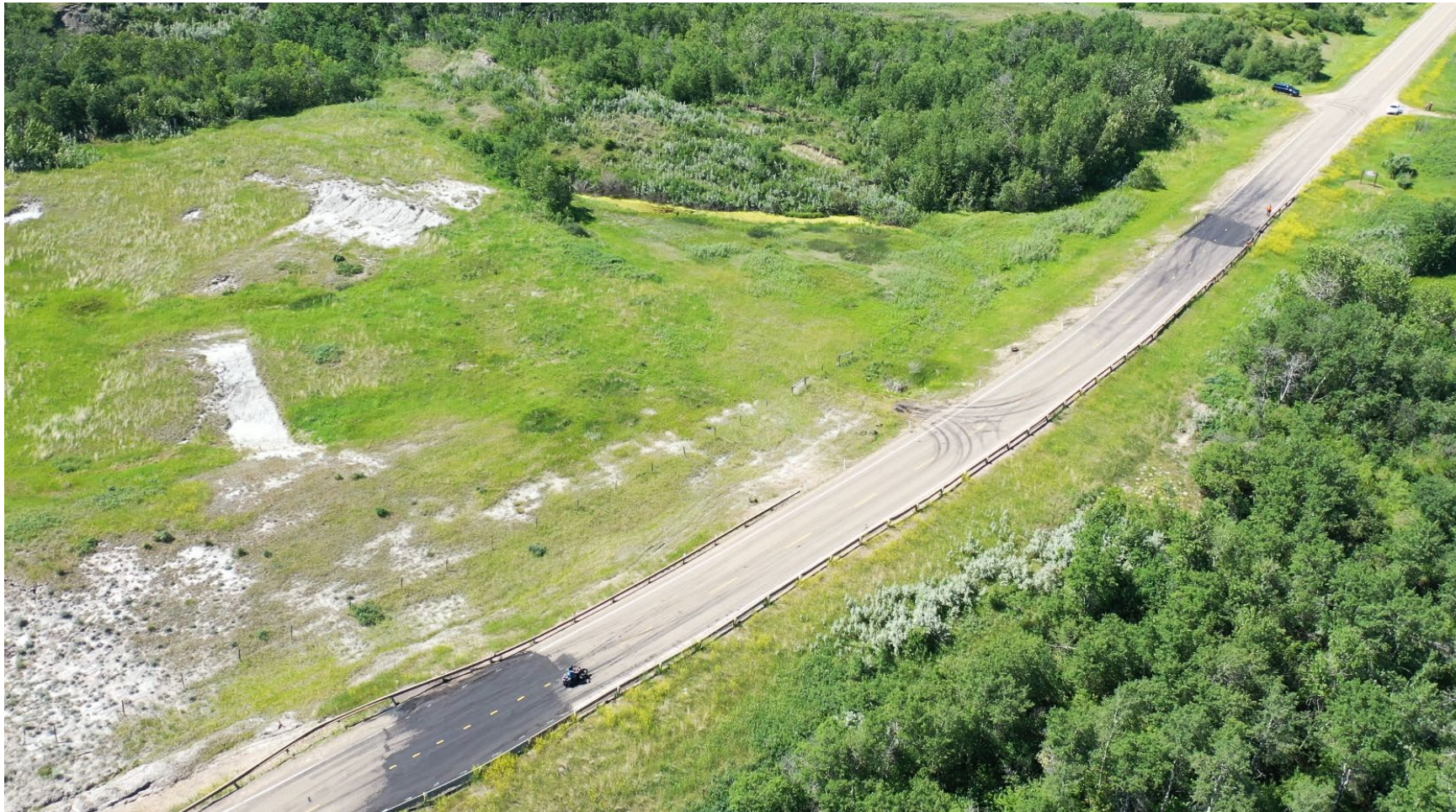
Photo 1 Oblique air photo of a portion of the C003 site, showing the guardrail deflection and two asphalt patches. Photo taken June 29, 2021 facing northwest.
