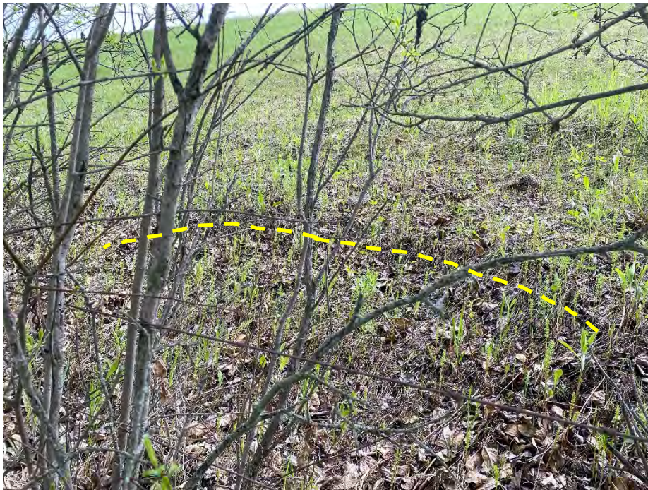
Photo 8: Old, vegetated ground crack near the north extent of the landslide zone. Looking northeast.
