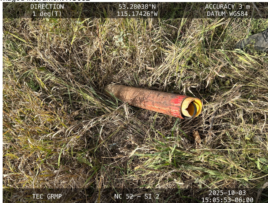
Photo 1: SI 2 sheared at approximately 0.72 m.
