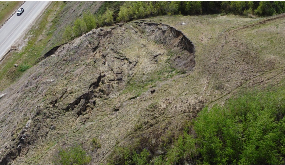
Aerial Photo 5: Looking northwest where landslide debris has been toppling over the edge of the steep bedrock slope
