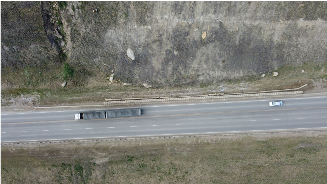
Aerial Photo 7: Few sandstone rock slabs accumulating behind the Concrete Jersey Barrier
