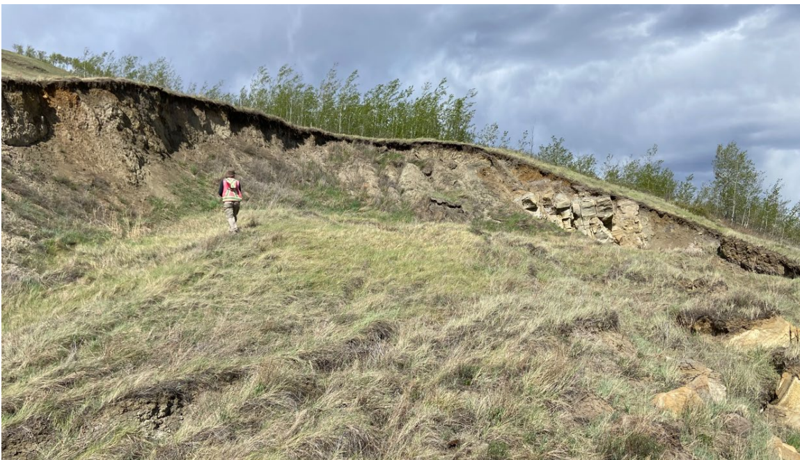
Photo 6: Landslide backscarp showing movements since 2023.
