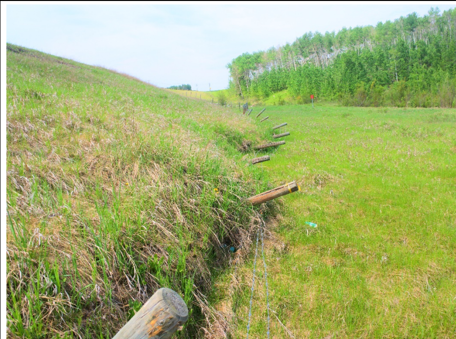
Photo 6. Looking northwest along the toe of the landslide. The fence posts are bent over further from movement of the toe bulge.
