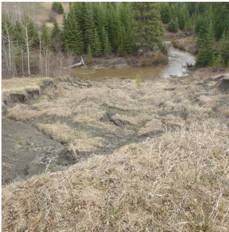
Photo 6 – Looking southeast at the outside bend of the river, which is causing the most active slumping area at Site 2.
