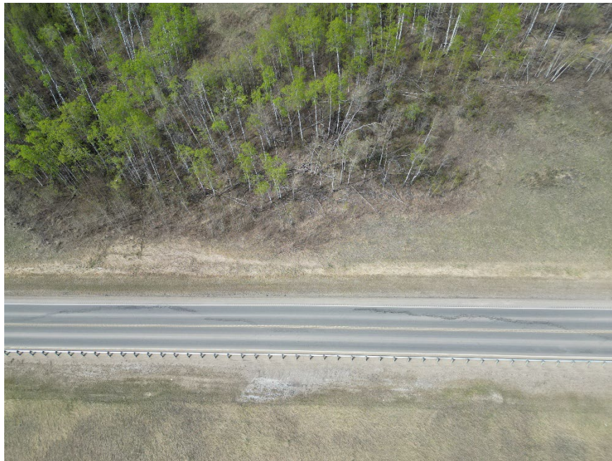
Photo 16. Drone looking north at the scarp crack near the west part of the site.
