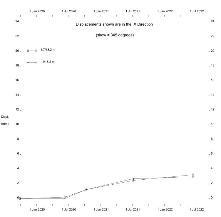
Hwy 740:02 Shaftesbury Trail, Inclinometer SI18-P30
