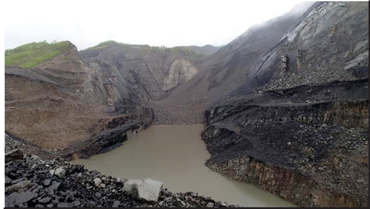
Photo 3a A settling pond inside the mine
