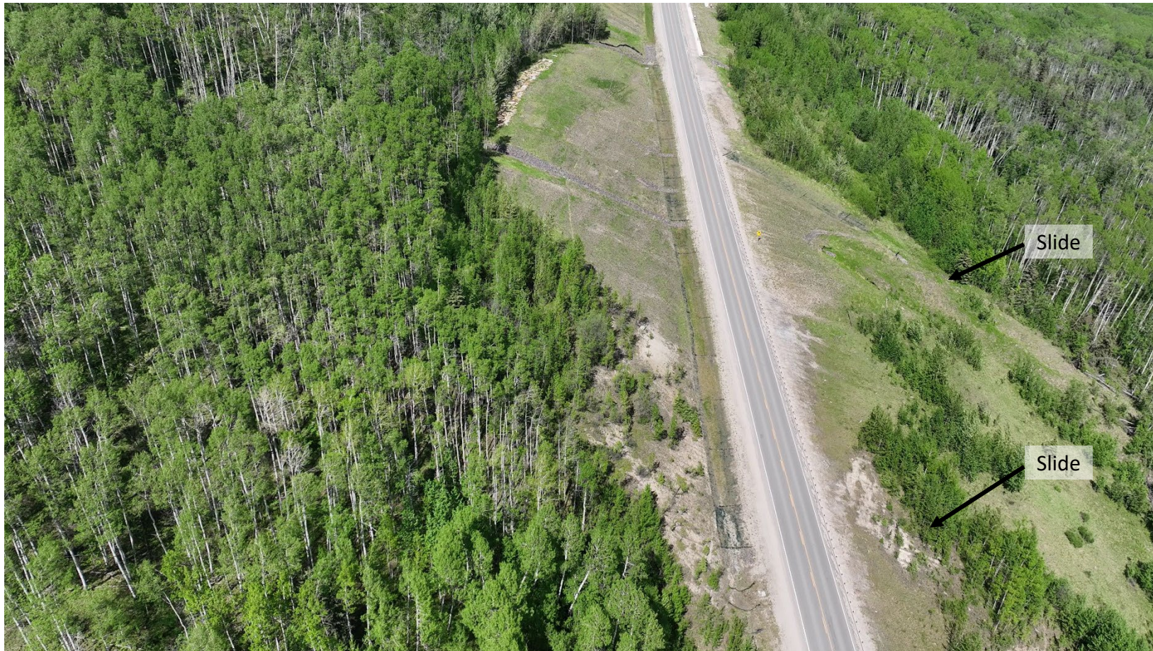
Photo 2 South portion of site. Note slides on east (downslope) side of Hwy 40:36. UAV photo taken June 2, 2025, facing northeast.
