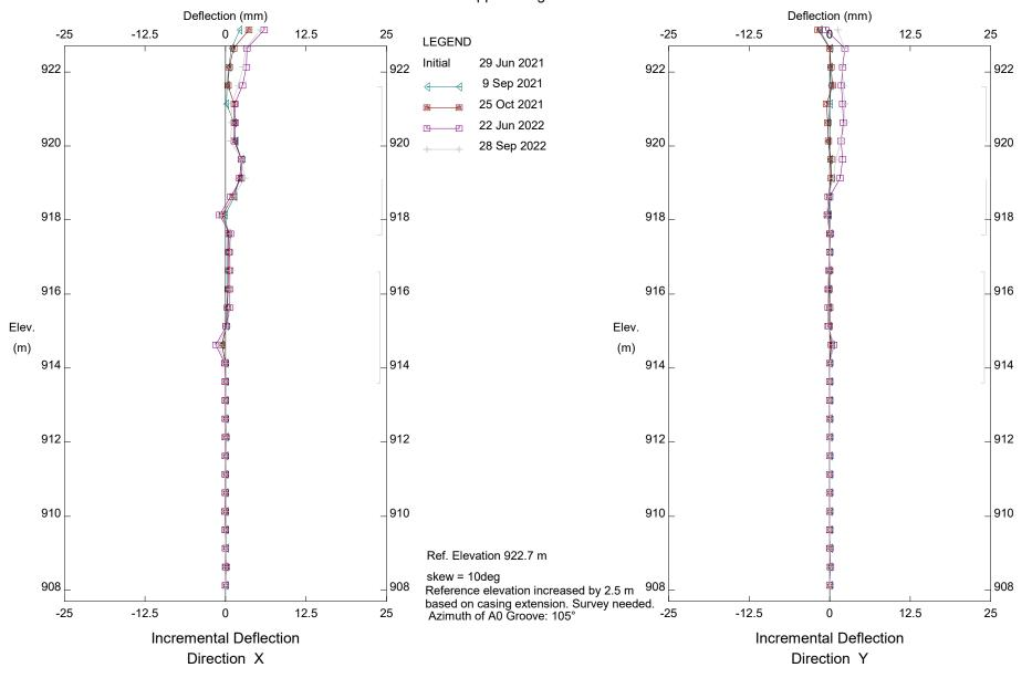
GP006; H40:36, Sheep Creek Embankment, Inclinometer SI-2
