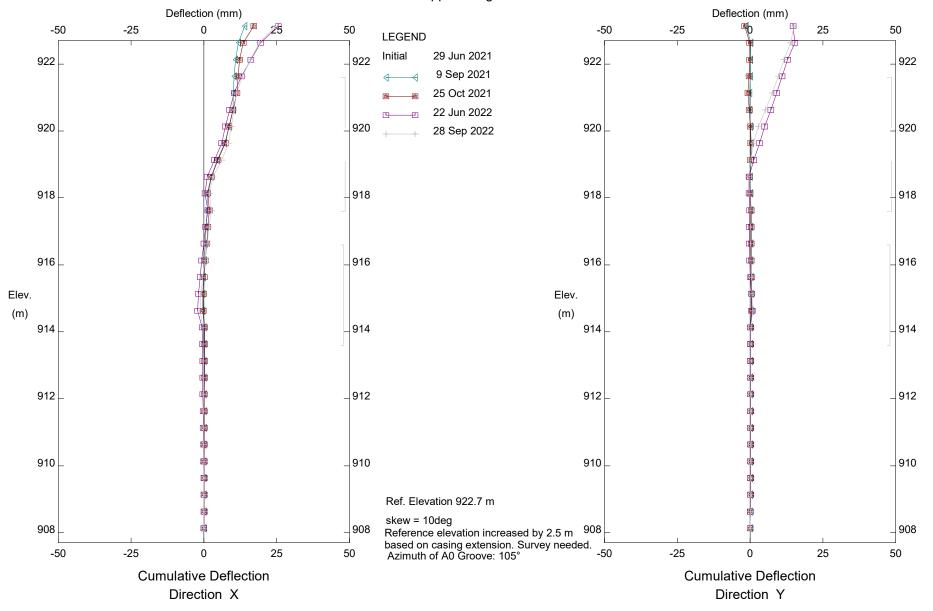
GP006; H40:36, Sheep Creek Embankment, Inclinometer SI-2
