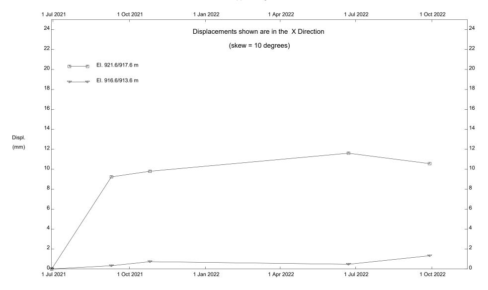
GP006; H40:36, Sheep Creek Embankment, Inclinometer SI-2
