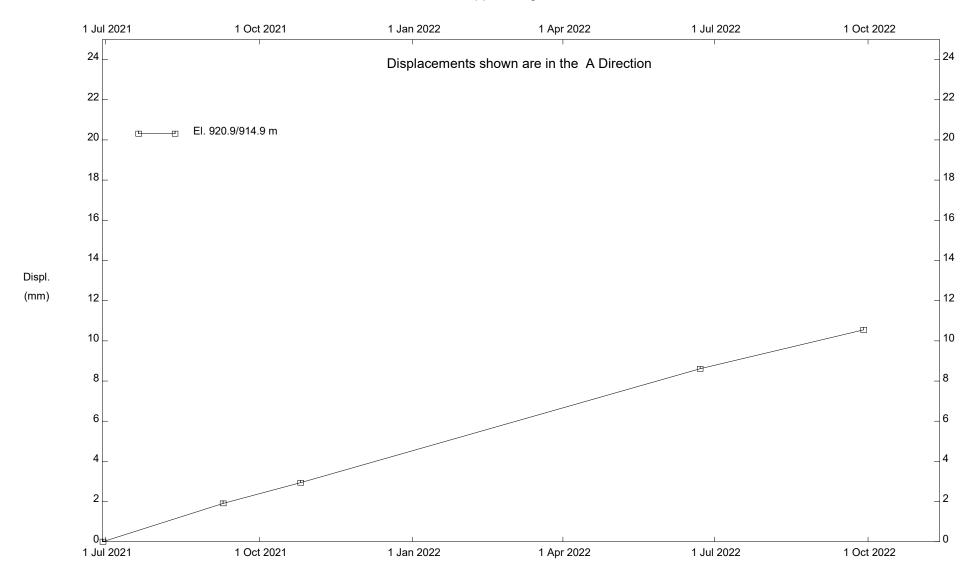
GP006; H40:36, Sheep Creek Embankment, Inclinometer SI19-2
