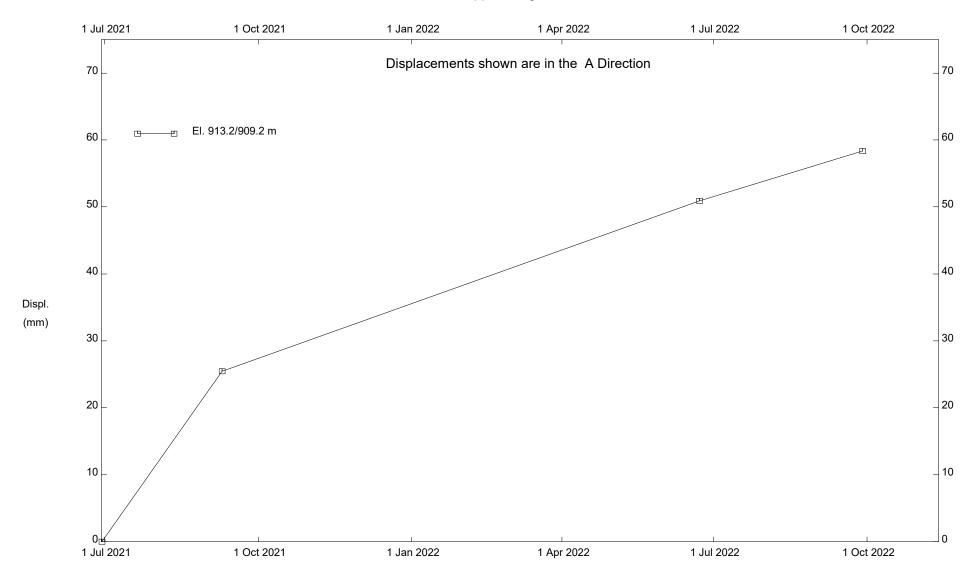
GP006; H40:36, Sheep Creek Embankment, Inclinometer SI19-3
