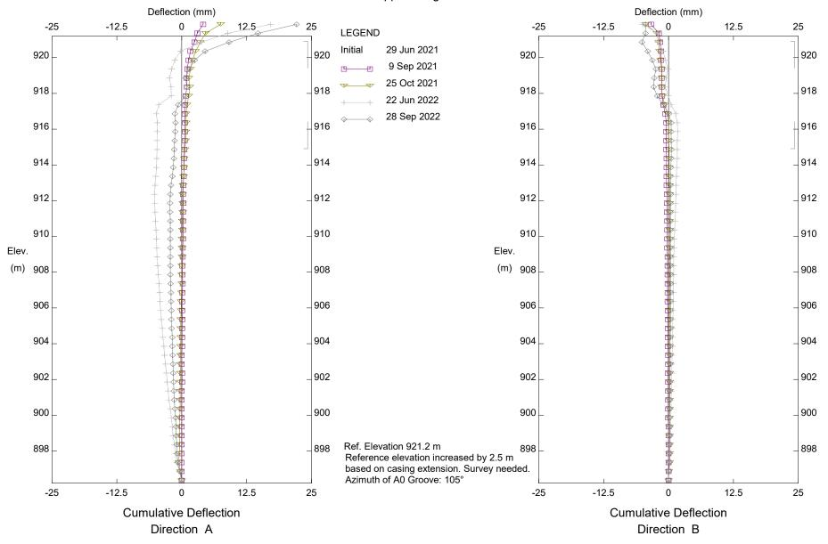
GP006; H40:36, Sheep Creek Embankment, Inclinometer SI19-2
