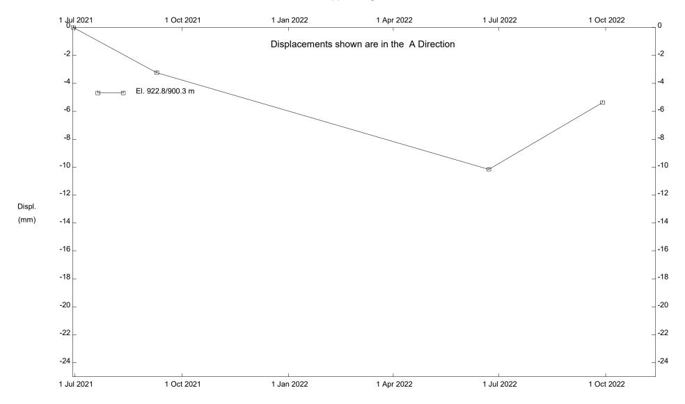
GP006; H40:36, Sheep Creek Embankment, Inclinometer SI19-1
