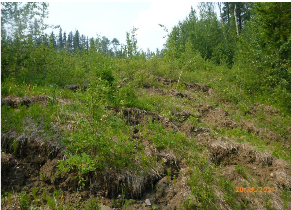
Photo 5 Cracking observed near the toe of the slide. Cracks were up to 0.5 m deep and filled with water (Waypoint 95 and 96). The slide appears more active at this area. Photo taken July 20, 2021 facing northwest.
