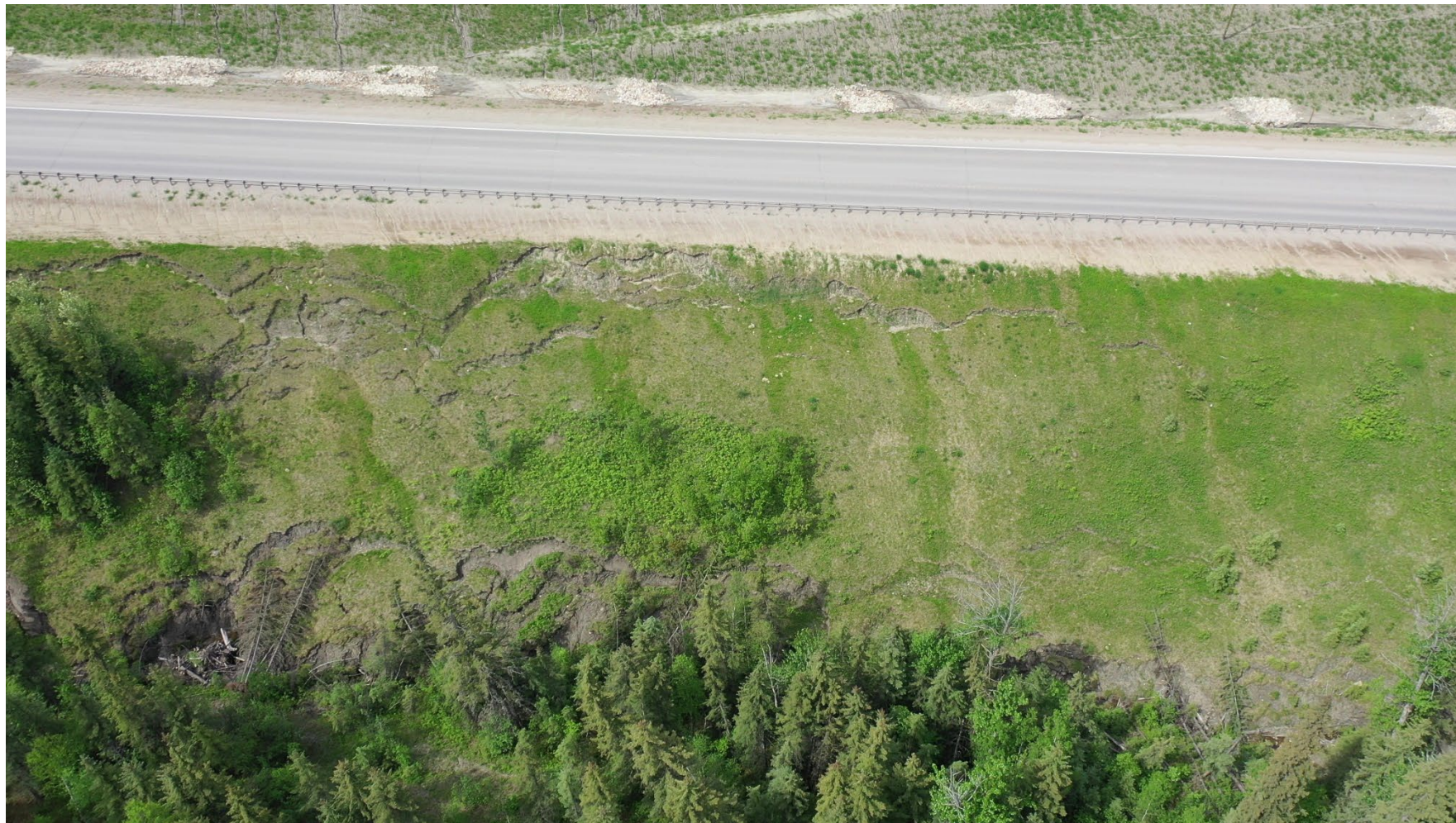
Photo 5 Series of slides between Hwy 40:38 and Roseham Creek. Photo taken June 15, 2022, with UAV facing west.
