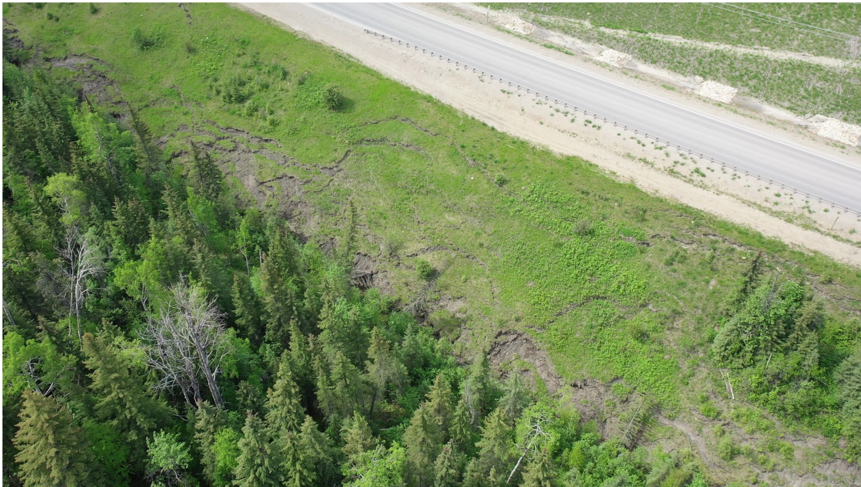
Photo 4 Series of slides between Hwy 40:38 and Roseham Creek. Photo taken June 15, 2022, with UAV facing southwest.
