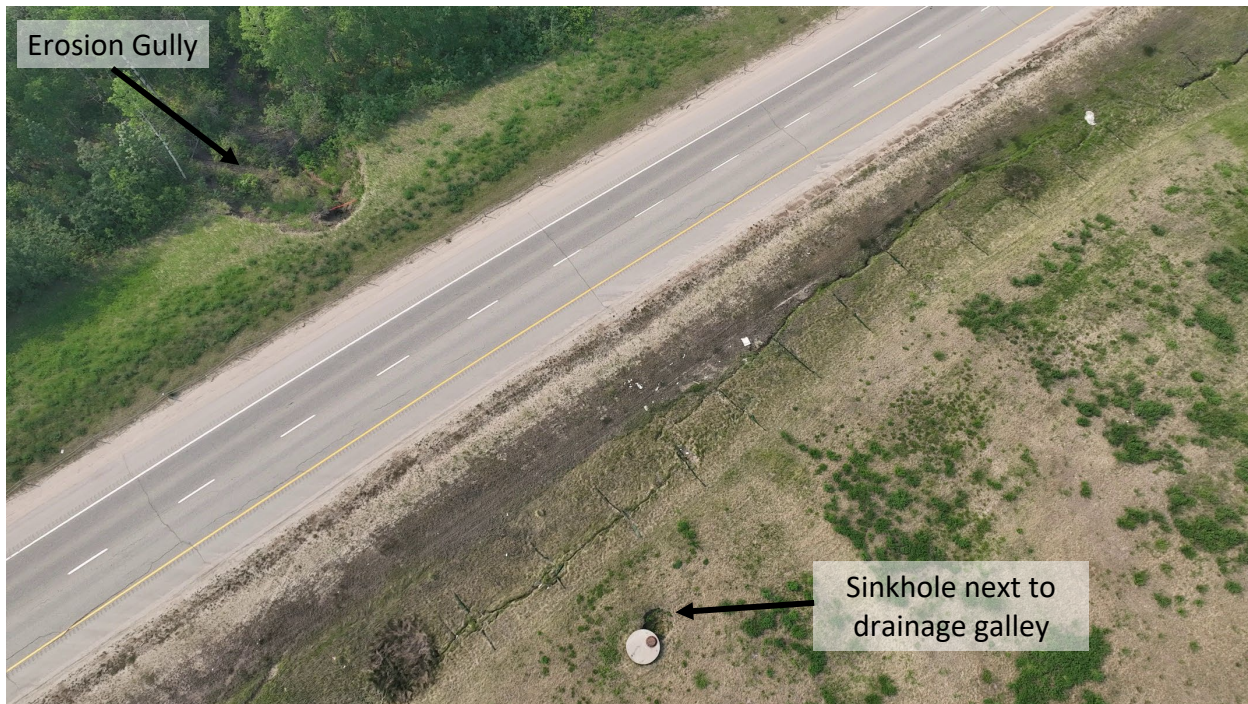
Photo 6 Erosion features in median backslope of Hwy 43:04. Photo taken June 3, 2025, facing southwest.
