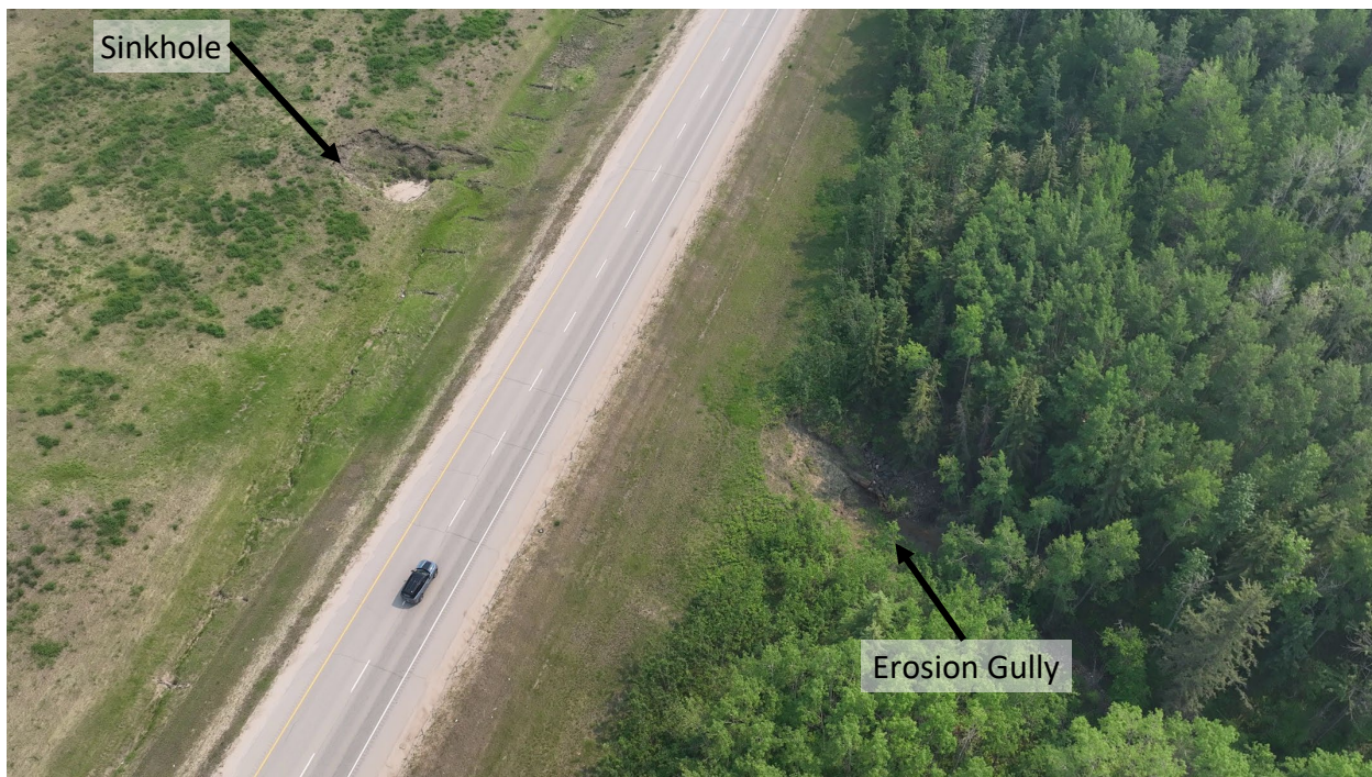
Photo 4 Sinkhole in median backslope and erosion gully on west slope of Hwy 43:04. Photo taken June 3, 2025.
