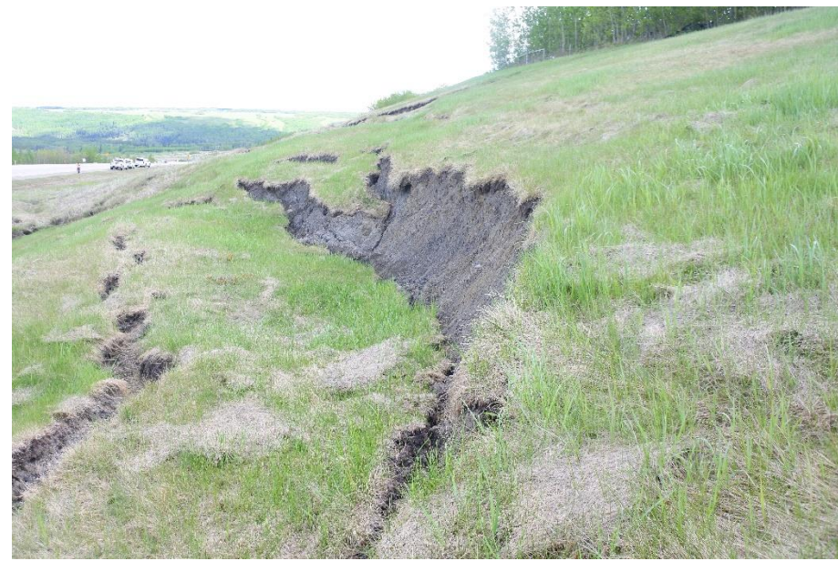
Photo 3. Looking southeast along the backscarp of Slide 1. The average drop along the backscarp in the western half of the slide is about 2.1 m in height.
