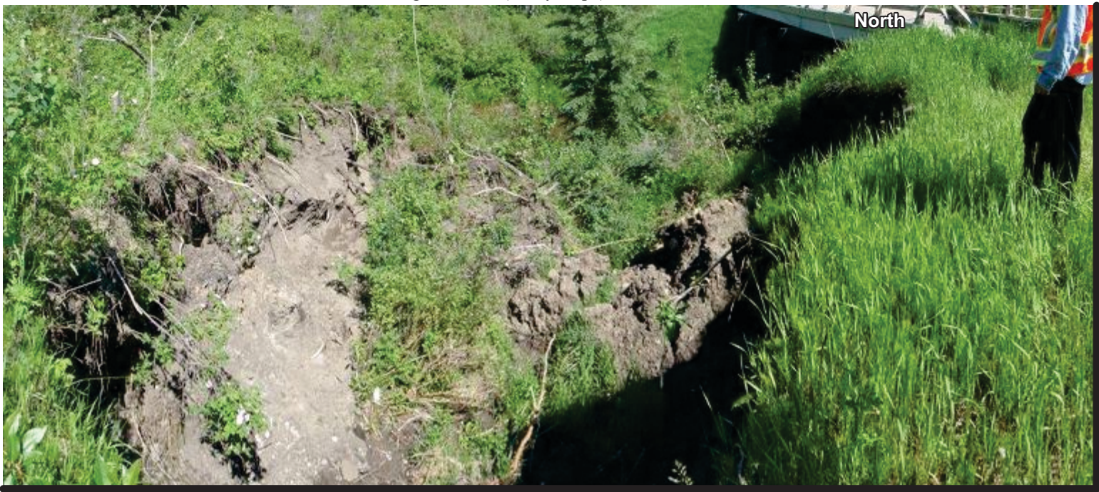
Photo IVa Looking north - down the head of slide • Powdery soil of weak strength and easily erodible
