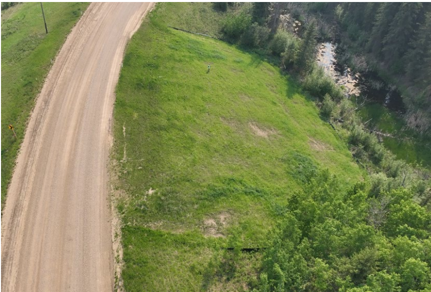
Photo 3 Repaired highway embankment slide on northwest side of Hwy 736:02. UAV photo taken June 3, 2025, facing southwest.
