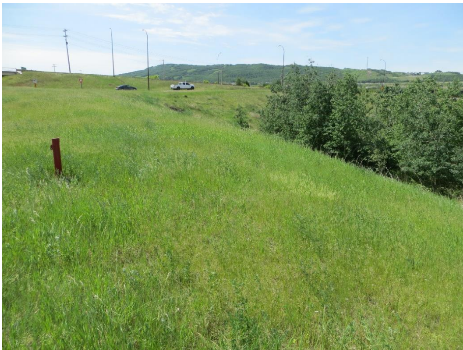
Photo 2. Looking south along the sideslope at the standpipe at the top of bank downslope of 98 Street. The standpipe is likely from test hole No. TH11-15 that was drilled as part of the geotechnical investigation by AECOM performed for the twinning in 2011.
