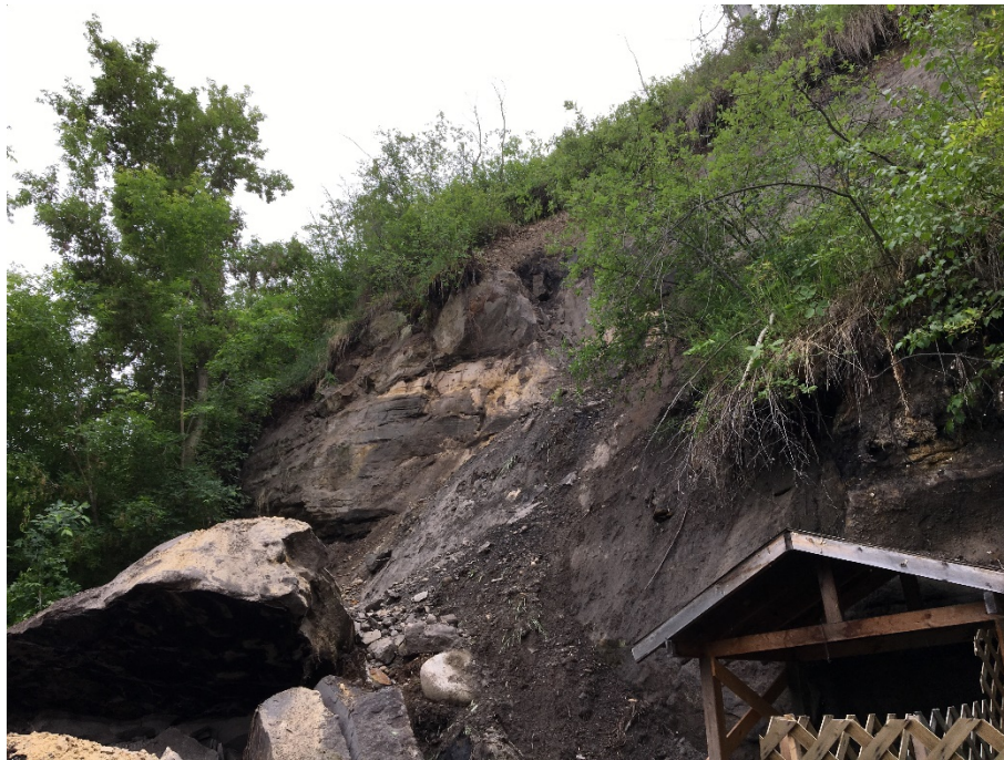
Photo 11: Looking southwest at upper weathered sandstone layer underlain by sand lens
