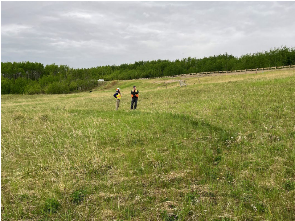
Photo 15 – Looking south at faint scarps observed downslope of highway.
