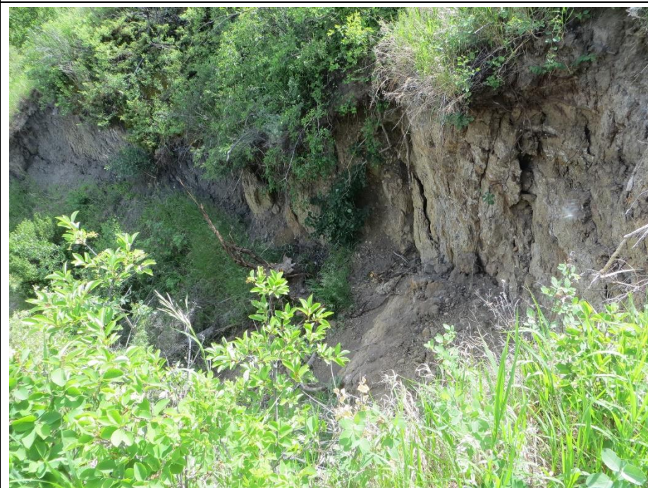
Photo 9. Looking southeast from the center of Slide 2. The south flank of the backscarp has been recently active with fresh debris accumulating below.
