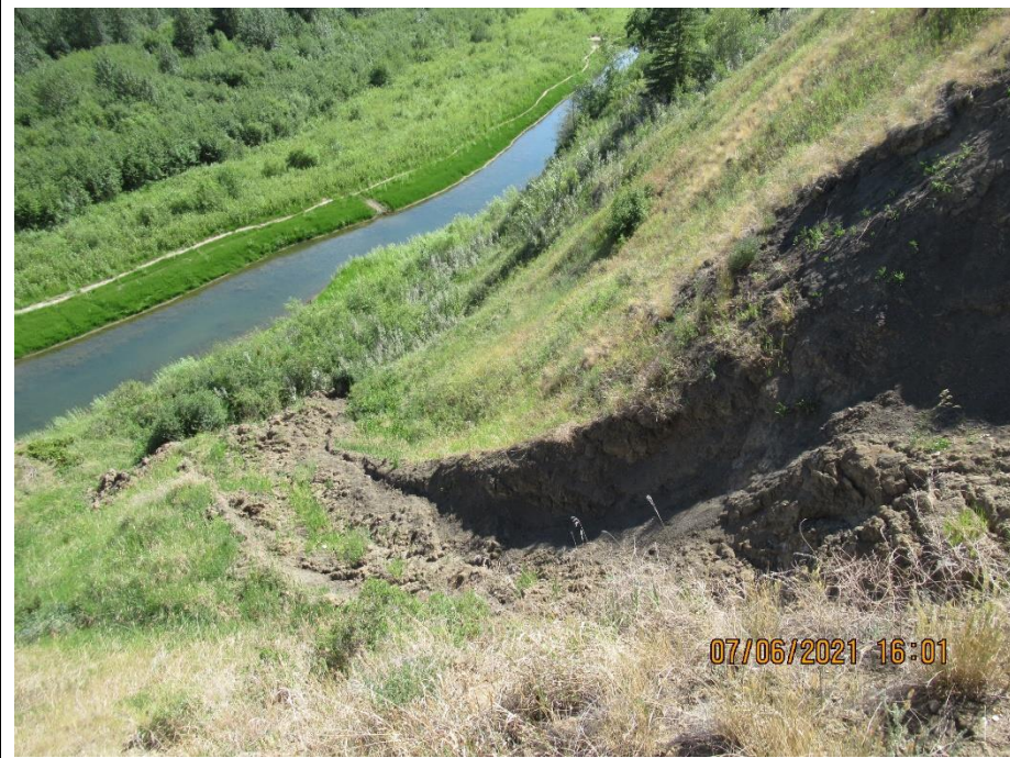
Photo 1. Looking south at the downslope area below the north side of Slide 1 at the mudflow at the base of the slide.
