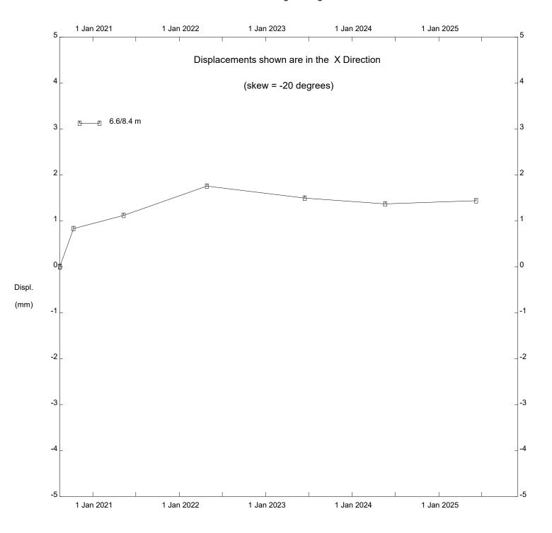
HWY 684 Shaftesbury trail, Inclinometer SI20-6
