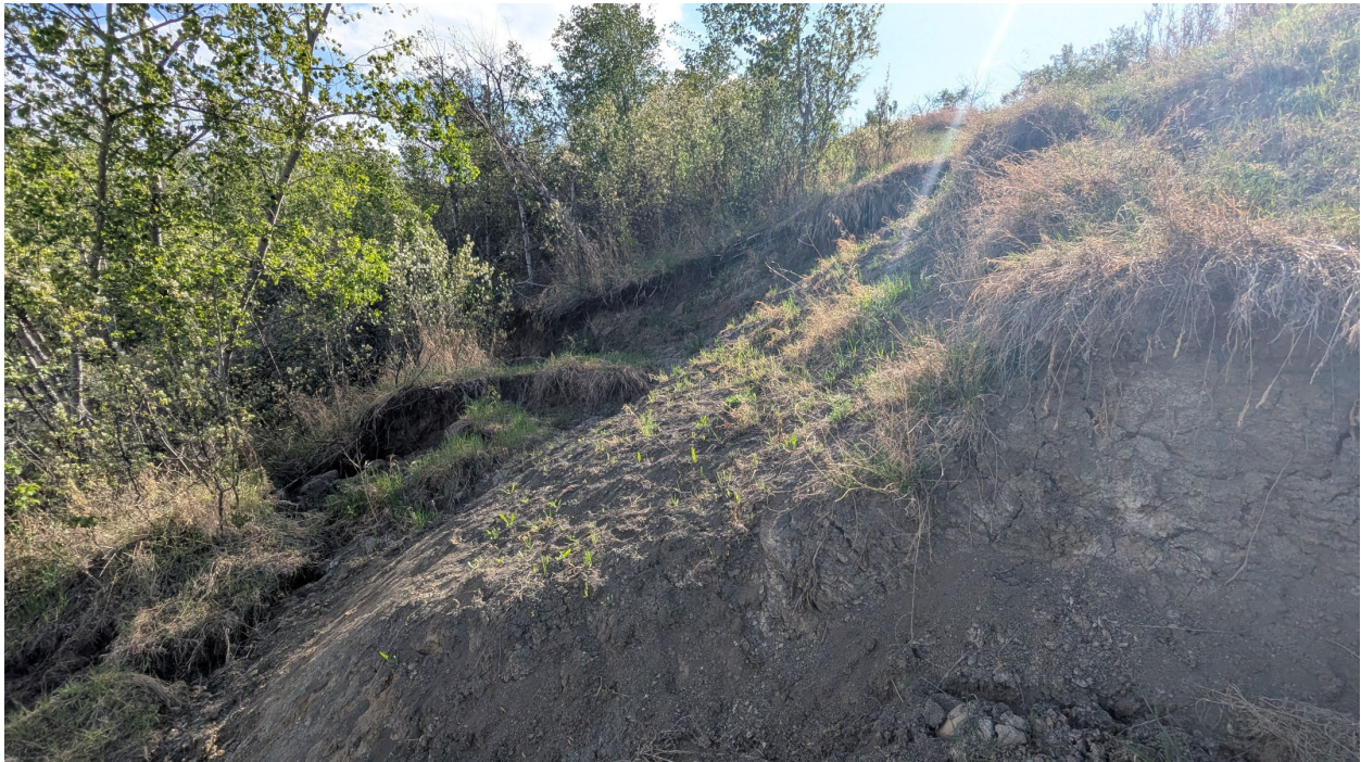
Photo 7: Additional scarps just beyond the west flank of the landslide. This is starting to move in 2025.
