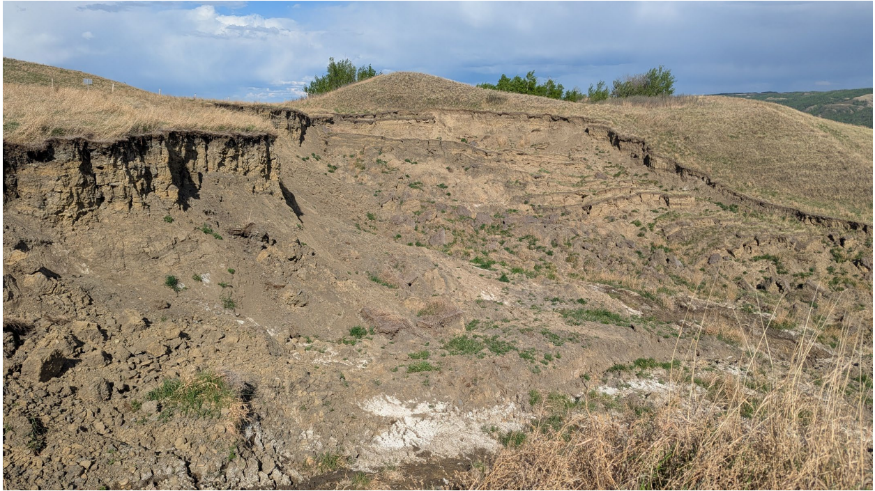
Photo 9: Toppling blocks at the face of the main headscarp.
