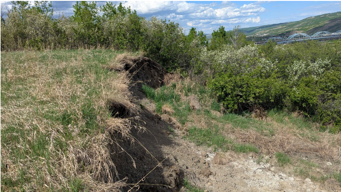
Photo 13: Looking north at the recent movement on the northwest flank of the active scarp. The CN rail line is located downslope of this landslide. The scarp has not retrogressed but the soil mass below has moved further downward.
