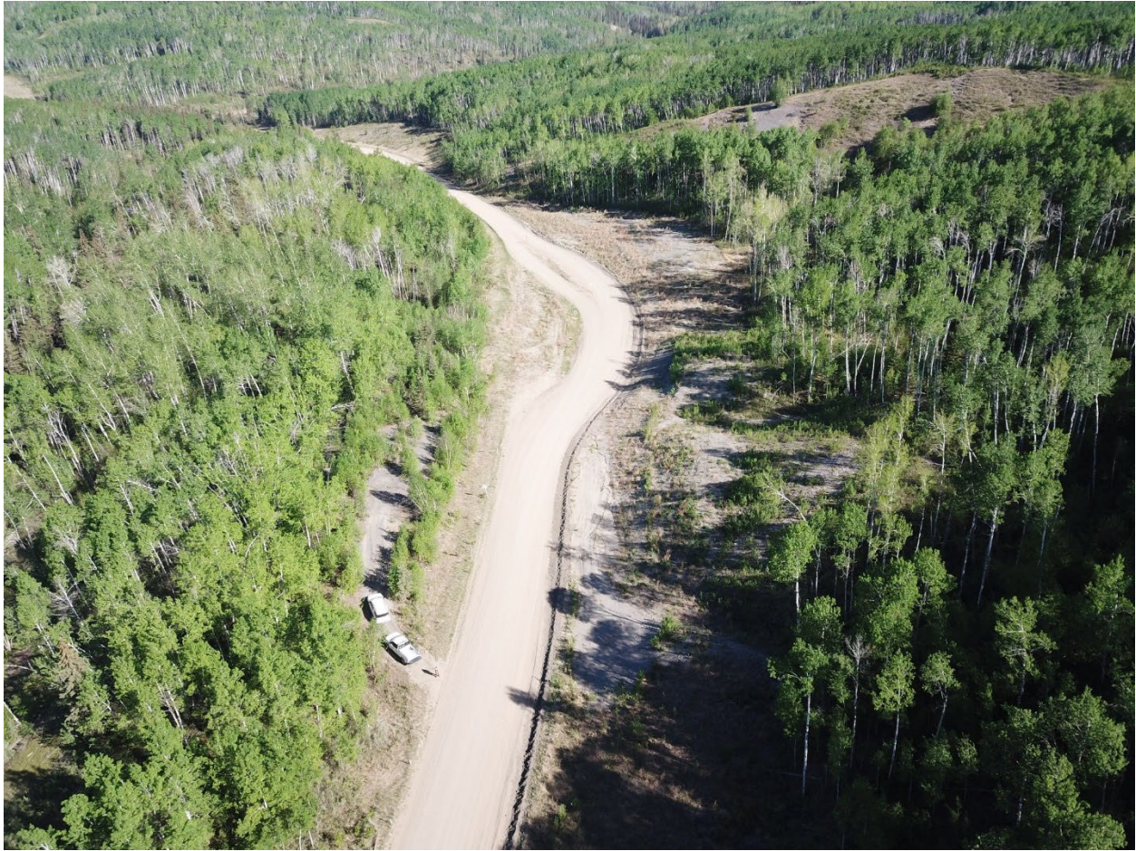
UAV Photo 2023 – Looking north toward the site: trucks are parked on the approach that was previously used for slumped soil from the PH011-2 backslope site. The bare area on the right side of the highway is where PH011-2 material has been spread recently. The detour around the slide is visible further north.
