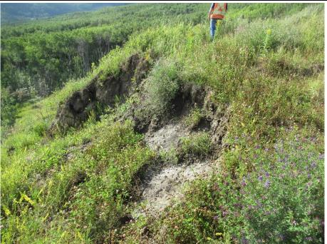
Photo 8. (Aug. 6/19) Looking southeast at some recent shallow movement in the native slope south of the sheet pile wall, below former slide 2.
