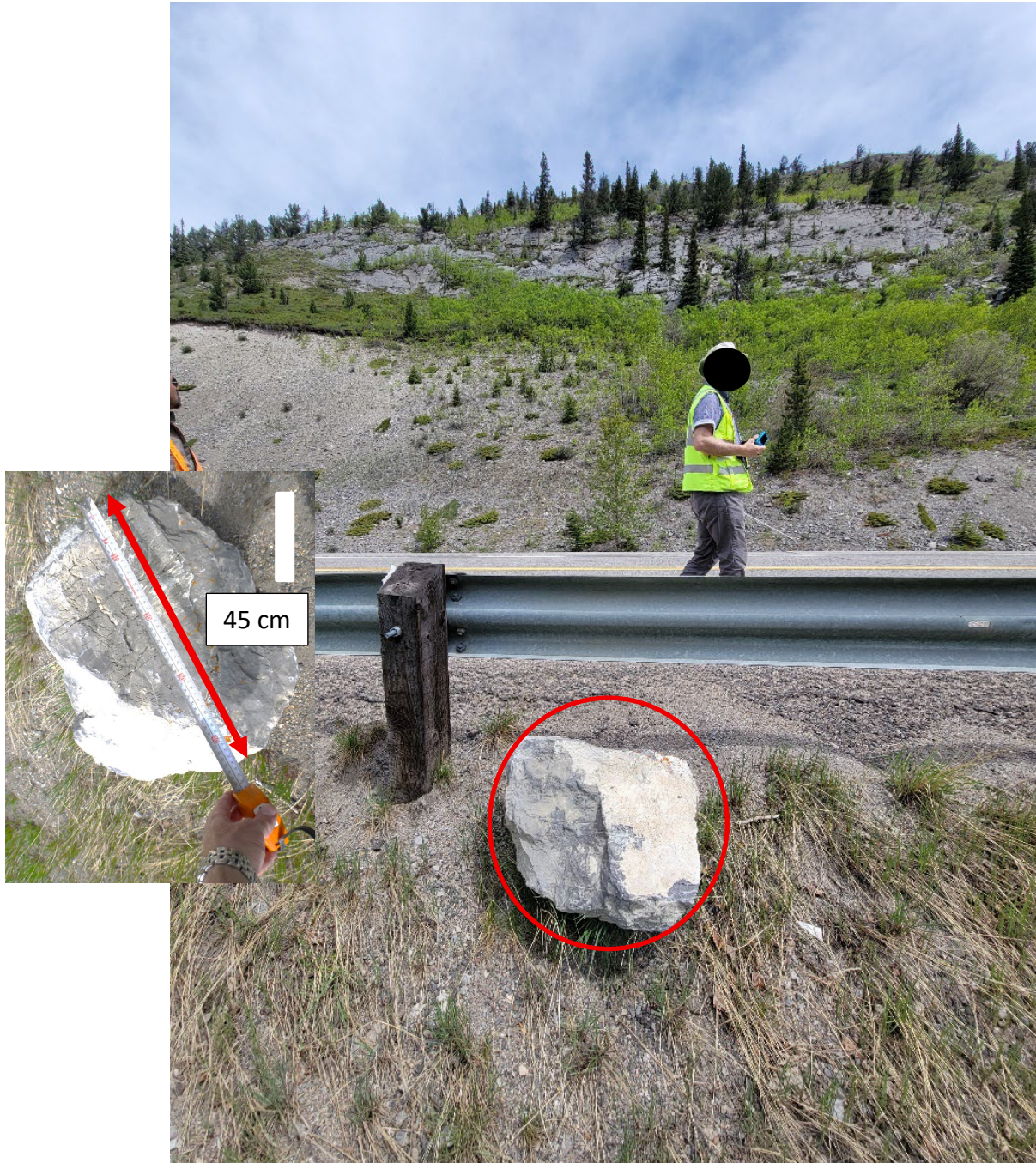
Photo 2 S070-2: Rockfall debris (red circle) on south side of highway which may have travelled across the highway. Photo taken facing northeast on May 27, 2025.
