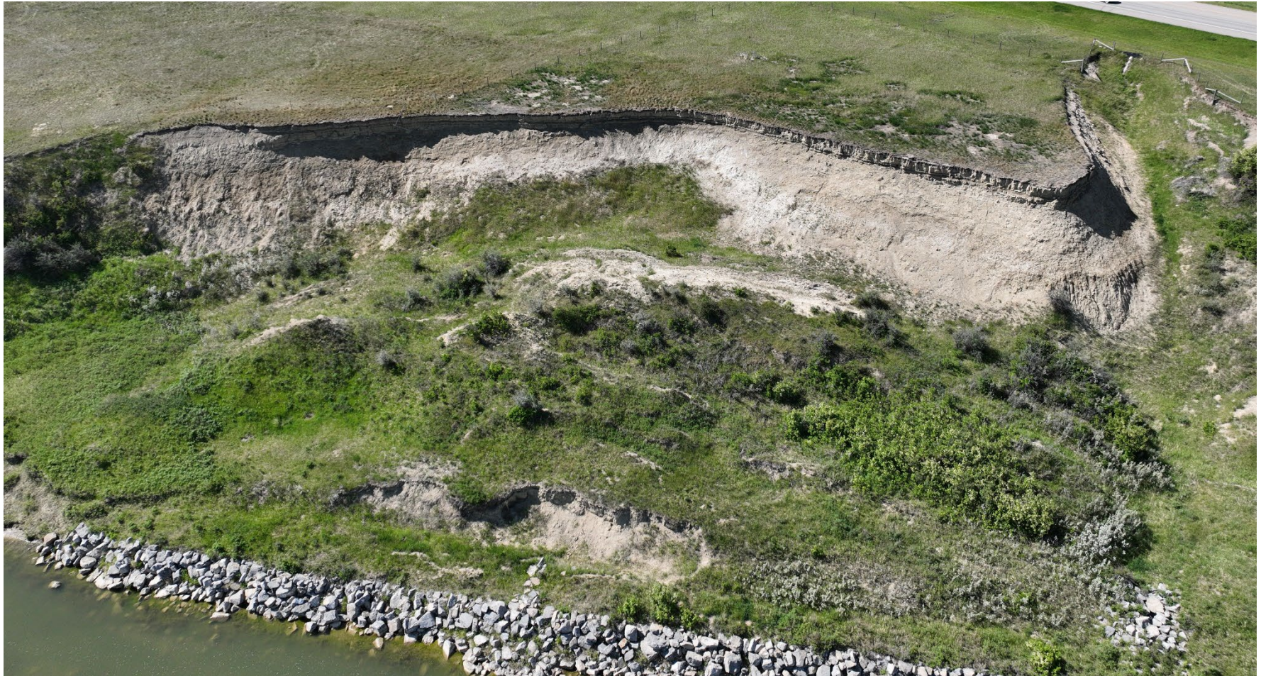
Photo 3 Aerial photo of the south extent of the site showing the steep unvegetated slope, culvert outlet, natural draw, and armoured shoreline. Photo taken May 28, 2025, facing southwest.
