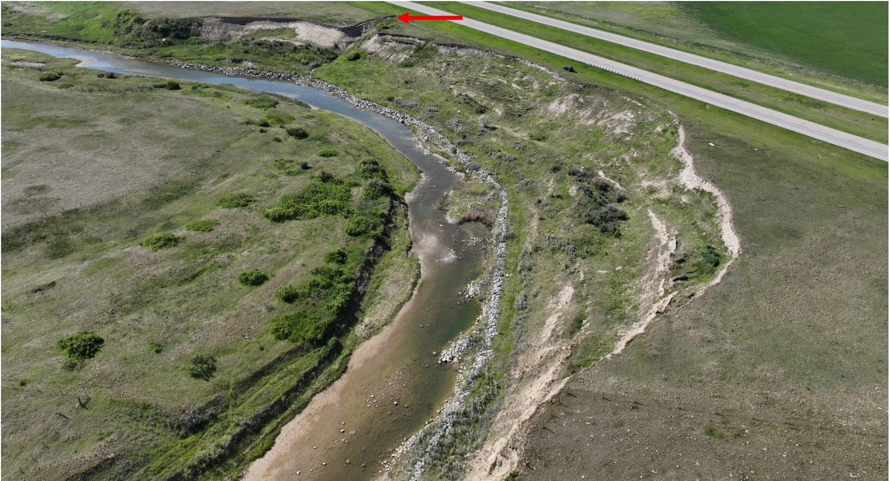
Photo 1 Aerial photo of the S004 site showing the slide extents, riprap armouring along the west shoreline of Willow Creek, and culvert outlet location (indicated by red arrow). Photo taken May 28, 2025, facing southwest.
