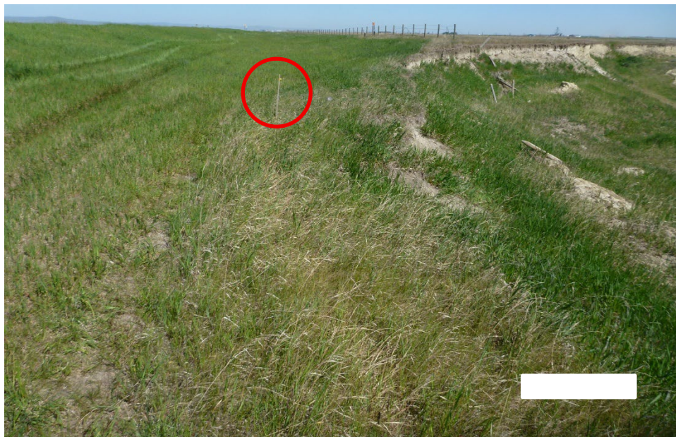
Photo 6 Wooden stake installed upslope of the slide (indicated by red circle) is approximately 1 m from the head scarp during the 2025 inspection. Photo taken May 28, 2025, facing north.
