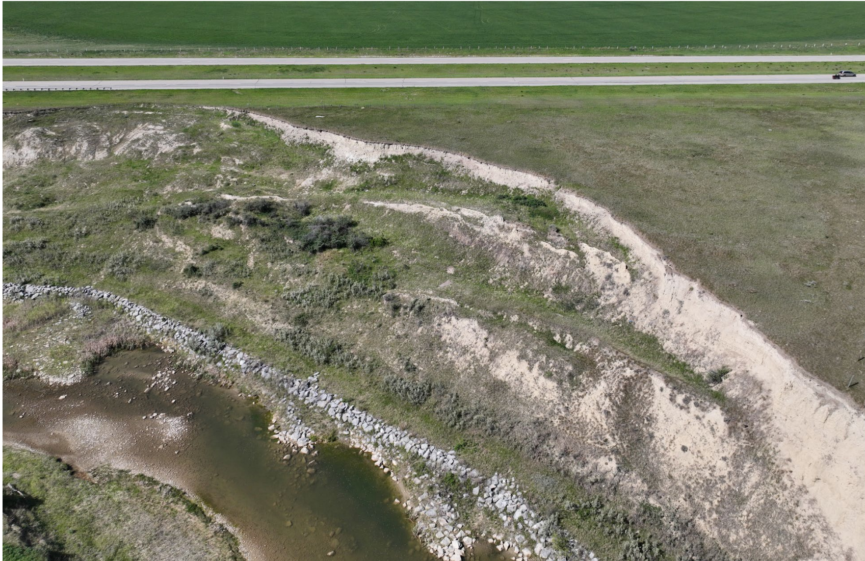
Photo 4 Aerial photo of the north extent of the site showing the steep unvegetated slope, natural draw, and armoured shoreline. Photo taken May 28, 2025, facing southwest.
