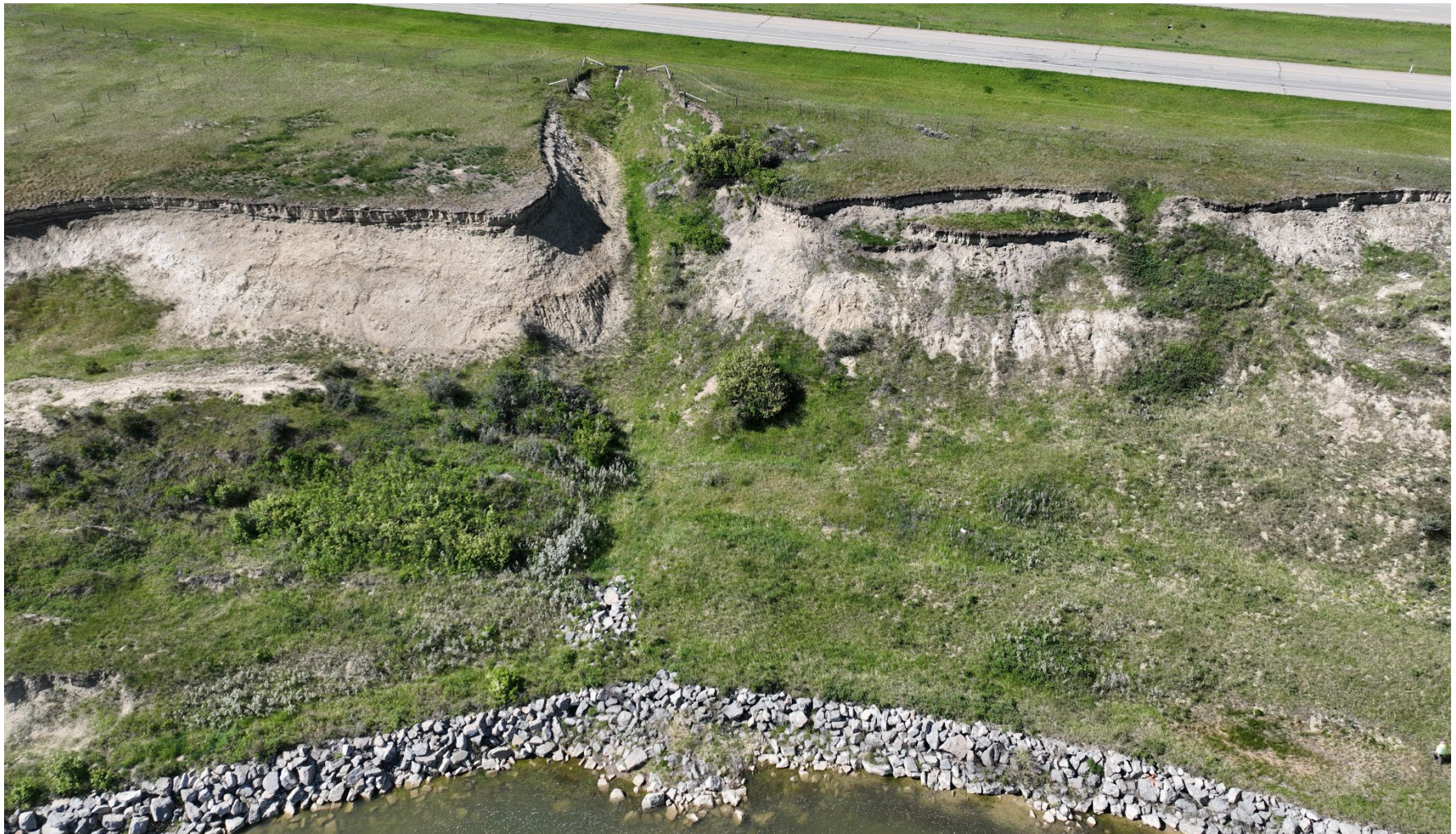
Photo 2 Aerial photo of the site showing the culvert outlet, natural draw, steep poorly vegetated slopes, and riprap armouring along the west shoreline of Willow Creek. Photo taken May 28, 2025, facing west-southwest.
