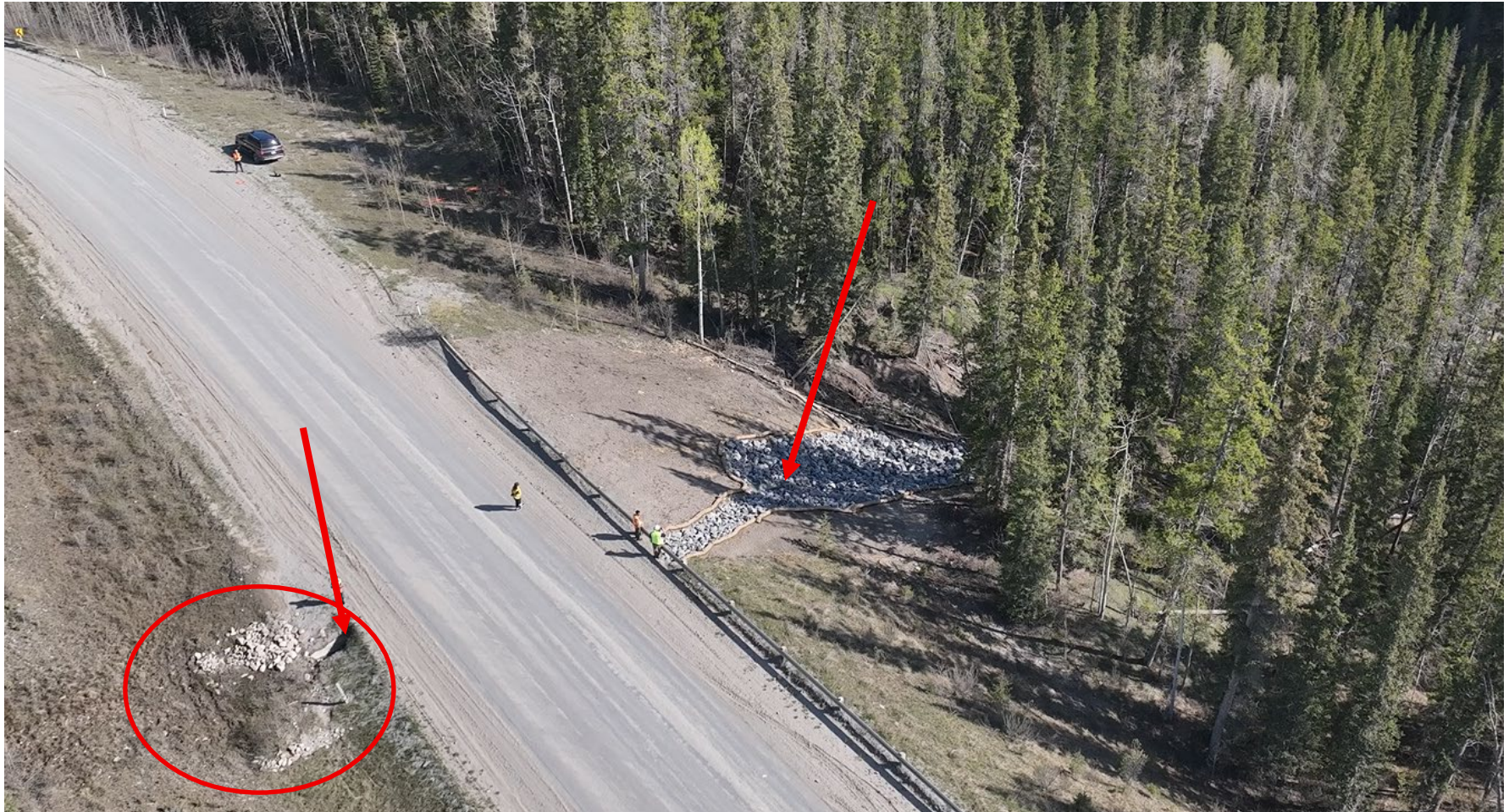
Photo 2 Aerial photo of the site showing the rebuilt slope, riprap armoured channels, and culvert outlet and inlet (indicated by red arrows). Two check dams of rounded cobbles and boulders are observed at the entrance of the culvert inlet (circle). Photo taken May 26, 2025, facing north.
