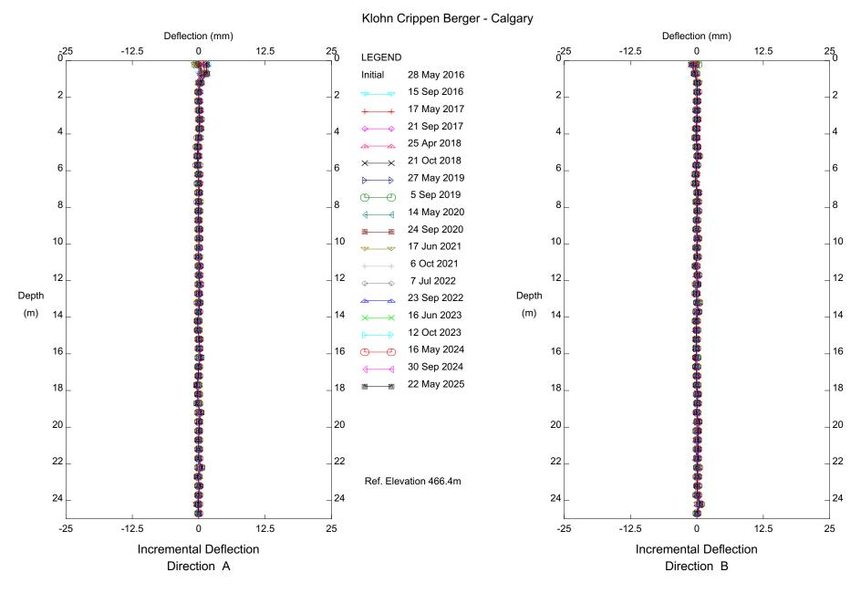
S026; H41:03, Elkwater Slides, Area A, Inclinometer Sl08-1
