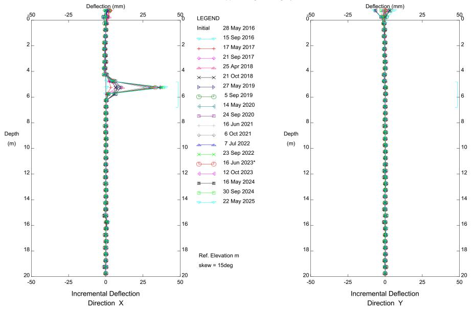
S026; H41:03, Elkwater Slides, Area B, Inclinometer SI12-01
