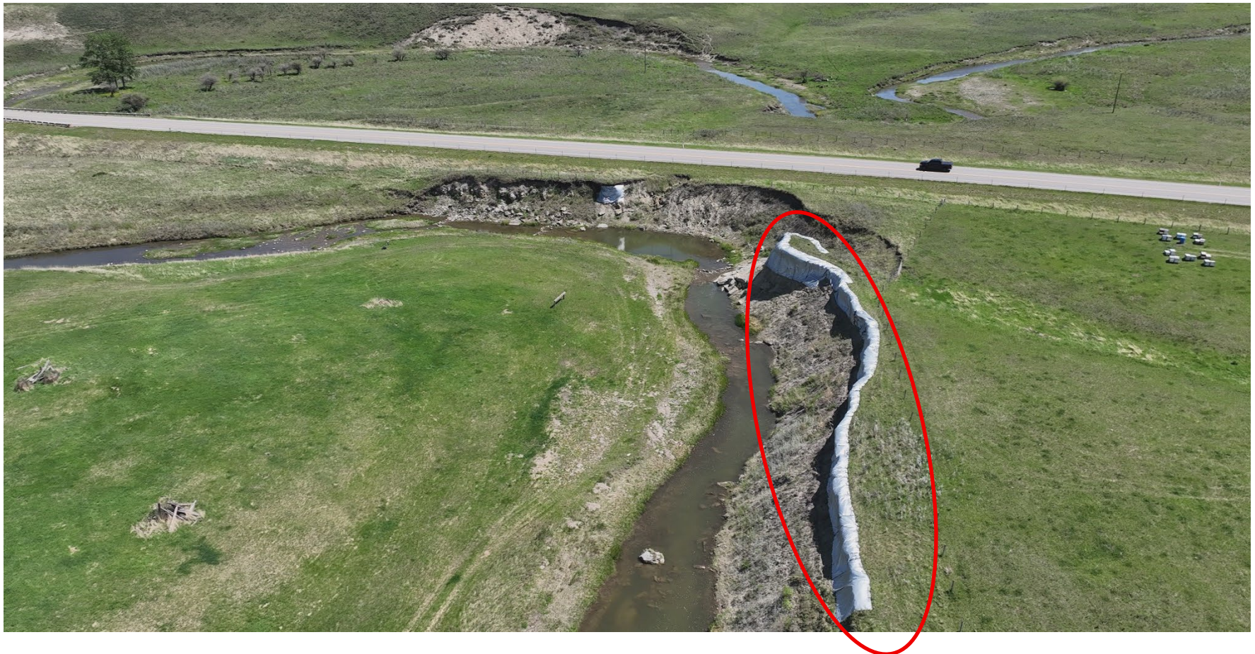
Photo 1 Aerial photo of the site highlighting Stimson Creek, erosion and slope instability, and tarps (red line) installed as part of bank swallow mitigation measures. Photo taken May 27, 2025, facing southeast.
