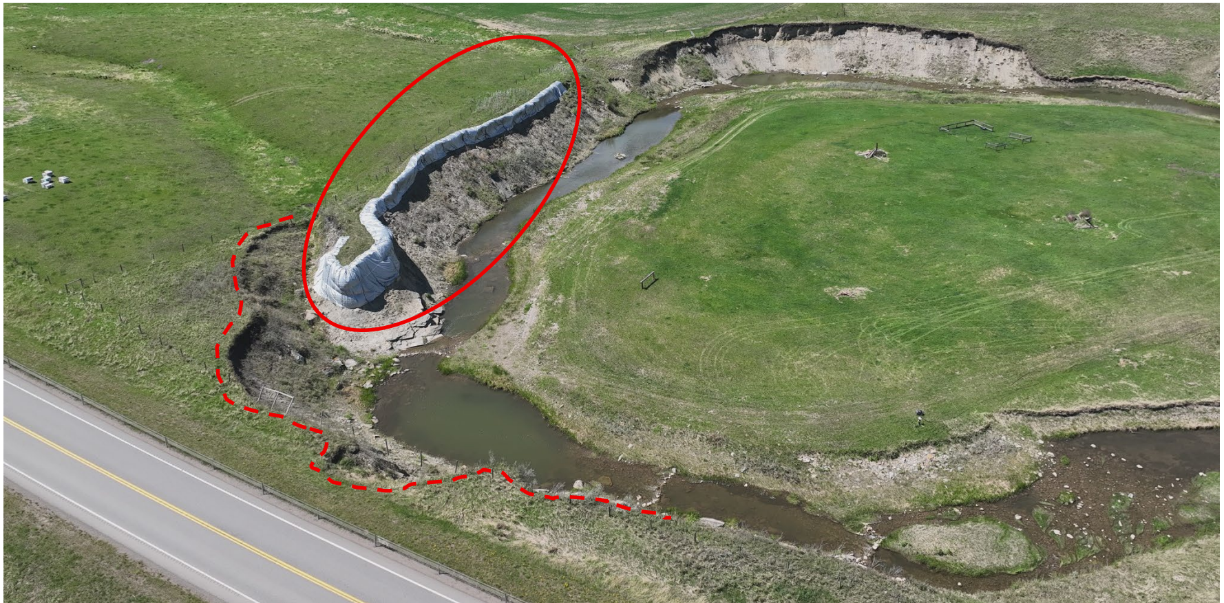
Photo 2 Aerial photo of the site highlighting Stimson Creek, erosion and slope instability (red dashed line), and tarps (red line) installed as part of bank swallow mitigation measures. Photo taken May 27, 2025, facing northwest.
