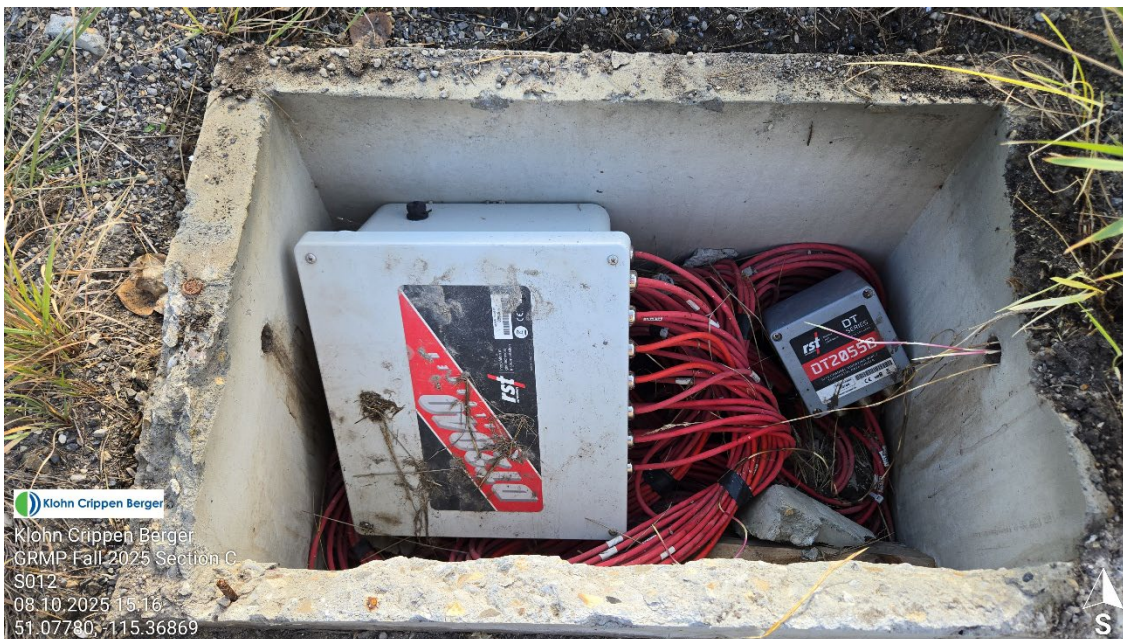
Photo 3.1 Damaged concrete enclosure where the data loggers are stored
