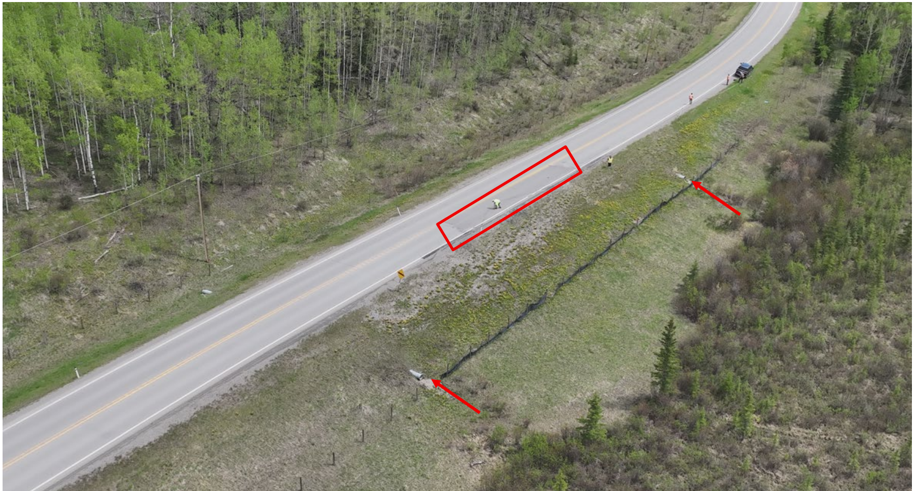
Photo 1 Aerial photo of the S031-2 site, highlighting the area of pavement distress (indicated by red rectangle) and culvert outlets (indicated by red arrows). Photo taken May 26, 2025, facing southeast.
