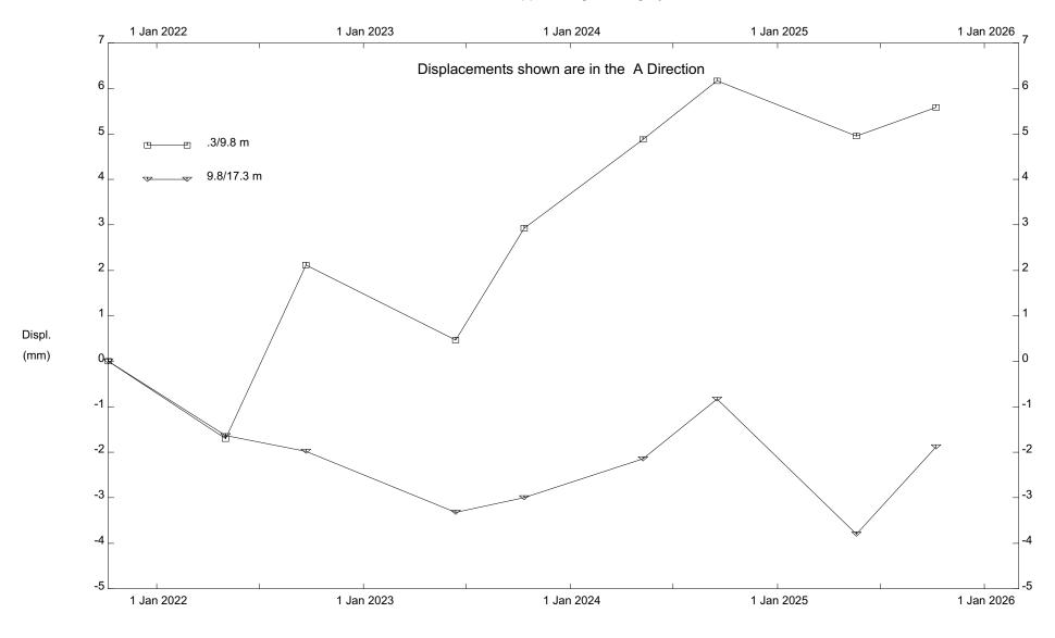
S008; H762:02, Fisher Creek, Inclinometer PILE15
