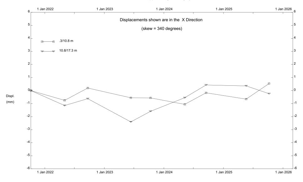
S008; H762:02, Fisher Creek, Inclinometer PILE36
