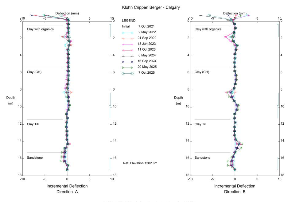
S008; H762:02, Fisher Creek, Inclinometer PILE15
