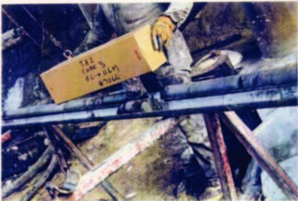
CORE SAMPLE : RUN 3 (8.6 - 11.6 m)
