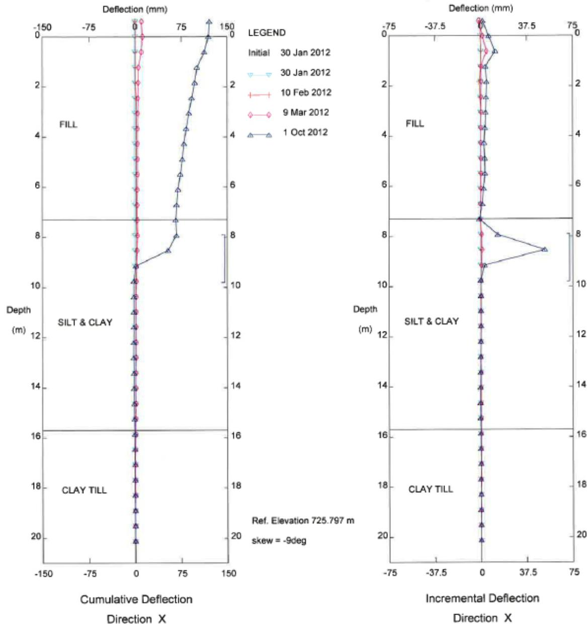
HWY 658:02 km 7.5 Blue Ridge Slide, Inclinometer SI12-3
