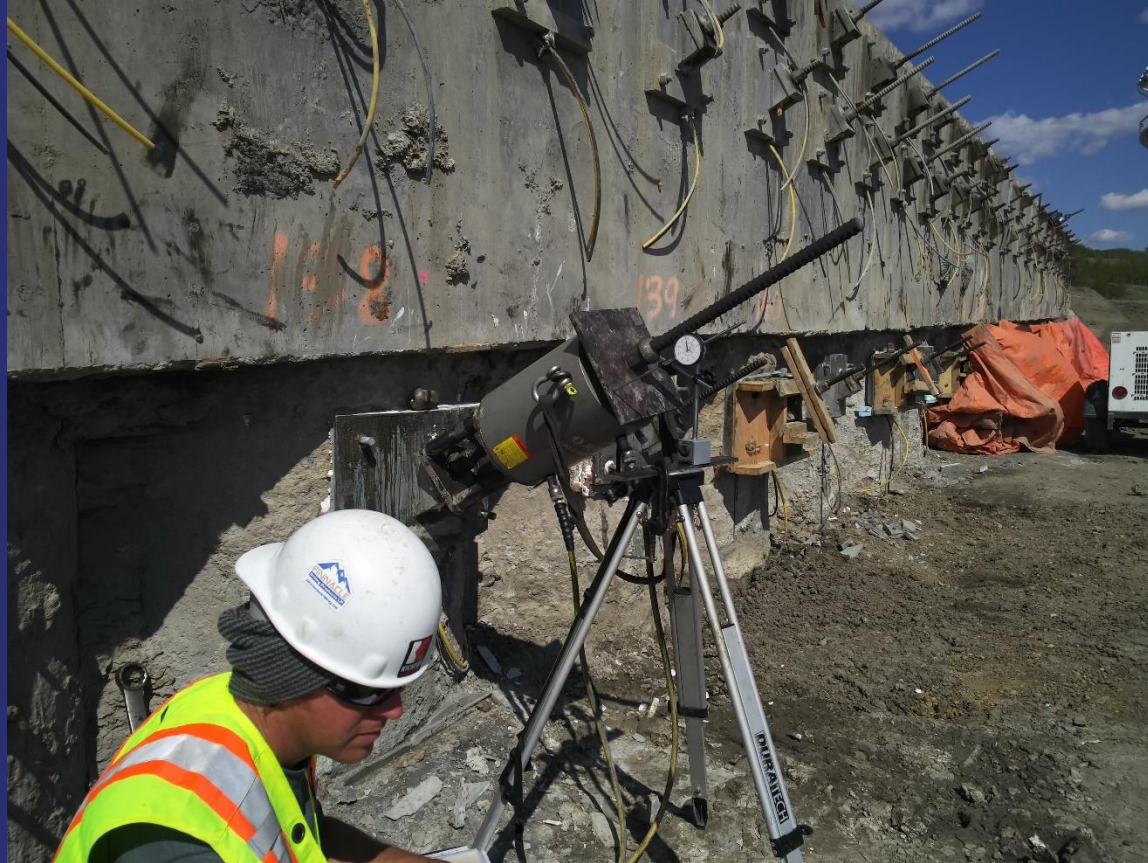
Wall Section 4 Pile Anchor Proof Testing
