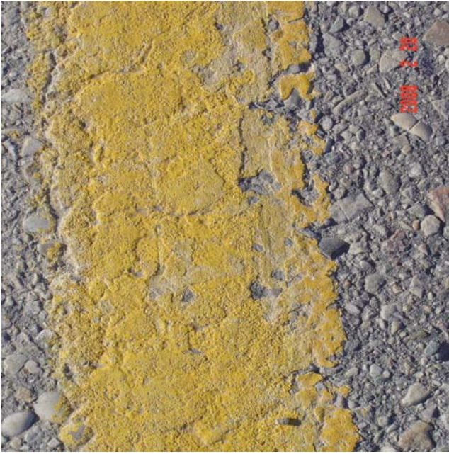
Yellow edge line: good durability, poor bead retention. Retro readings: 49, 46, 43, 52, 49, 49, 51, 45, 52, 43, 47, 47 Average: 44 Mcd
