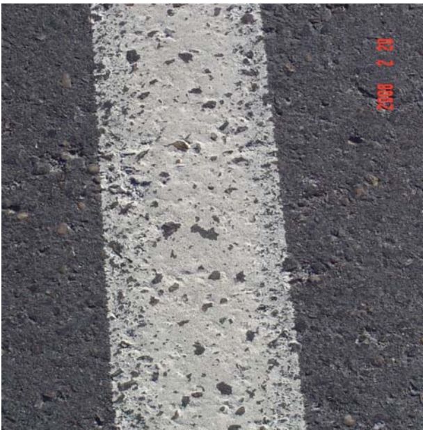
White edge line: paint chipping, loss of bead Retro readings: 65, 71, 62, 66, 76, 72, 64, 77, 67, 64, 72, 74 Average: 92 Mcd
