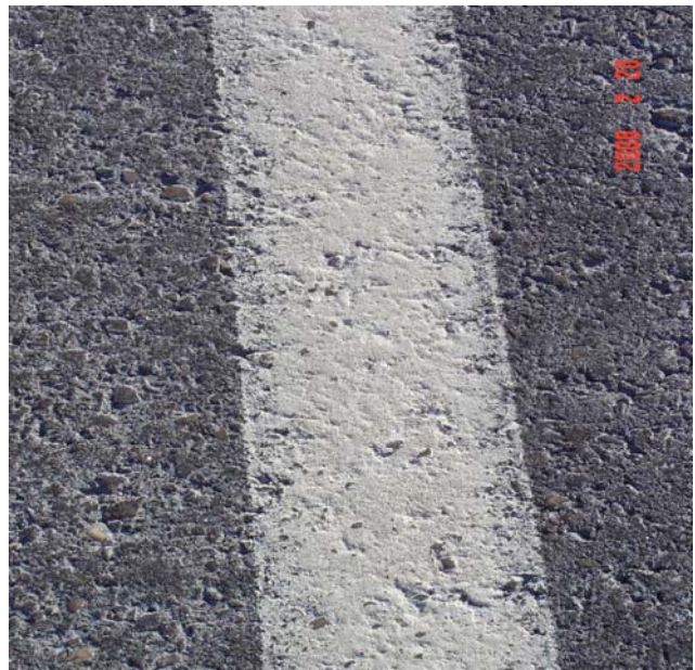
White skip line: good appearance and bead retention Retro readings: 93, 86, 105, 92, 112, 102, 102, 112, 111, 94, 111 Average: 93
