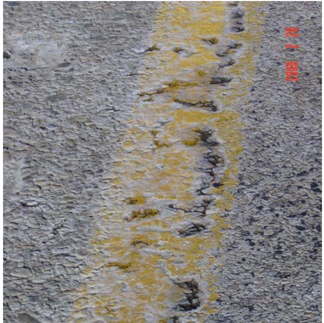
Yellow edge line: more snowplow scapping at this location, however good bead retention. Retro readings: 107, 124, 109, 103, 97, 93, 105, 122, 122, 93 –
