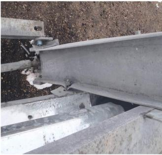
Post slightly twisted at end (notice tear at bolt location)
