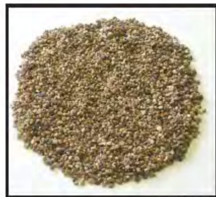
Very coarse sand makes for the best backfill.
