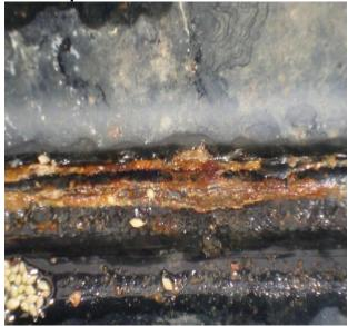
Corrosion at the lock seam seam location
