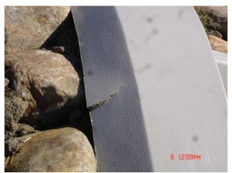
Close-up, showing tear in fibreglass (downstream end)
