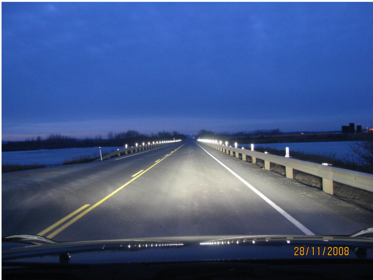
Hwy 619:06 Test Section 15" Guardrail Reflectors - Highbeam (Note: smaller current reflectors still in place)
