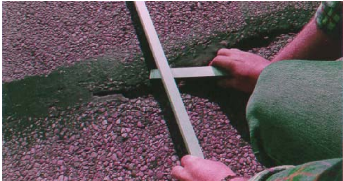
INCORRECT - Do Not Drop The Wedge Down Into The Crack, Reading Will Be Exaggerated
