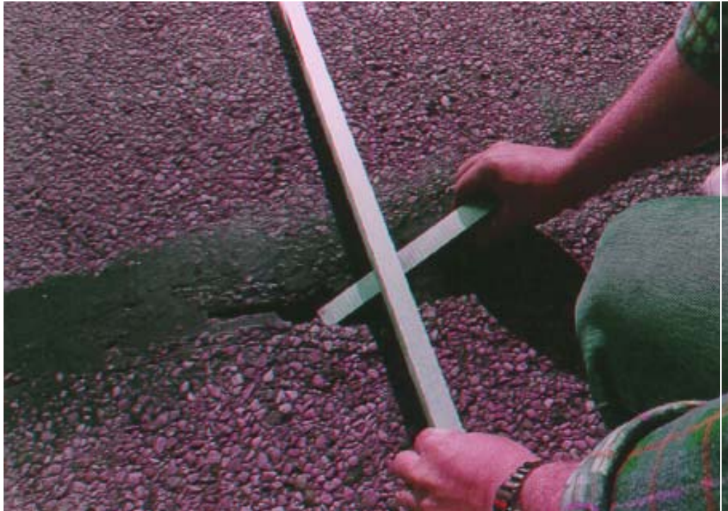
INCORRECT - Do Not Drop The Wedge Down Into The Crack, Reading Will Be Exaggerated
