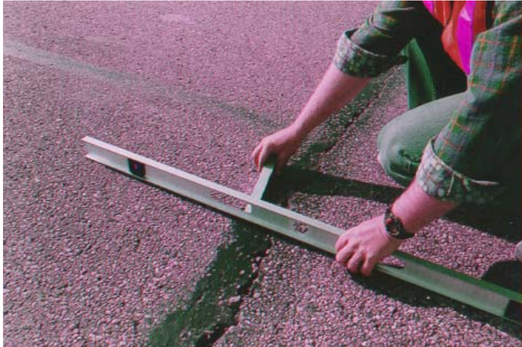
INCORRECT - This Reading Will Not Produce The Maximum Depression
