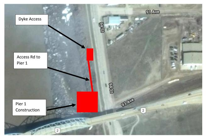
This new access through the dyke includes a monitoring plan that was put in place to adapt quickly to changing river conditions. Equipment and material are on site to reinstate the dyke within hours if river conditions change. It's estimated to take between six to eight hours to reinstate the dyke.
