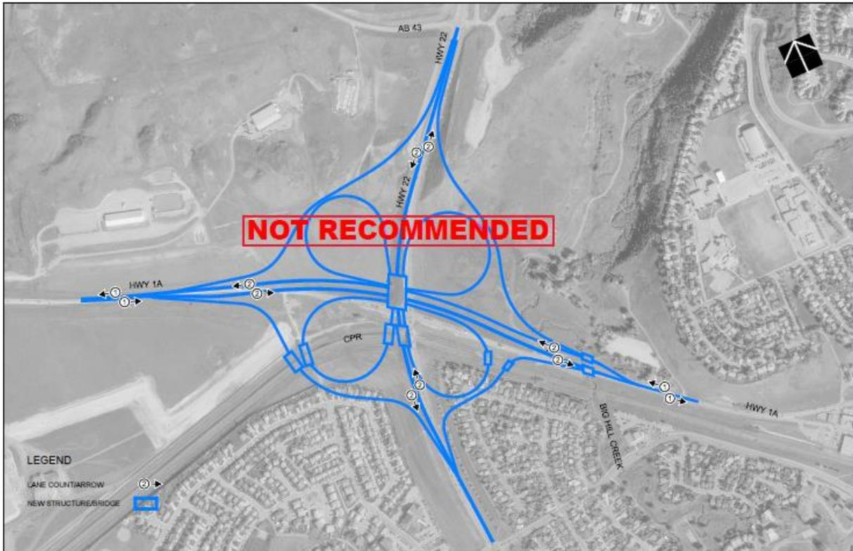
Cloverleaf configurations are not commonly built anymore due to short acceleration/deceleration distance between the loops, which becomes problematic and less safe with higher traffic volumes and it has a larger footprint than other options.
