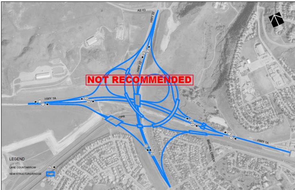
Building a “free flow” interchange with flyover ramps would require significantly more land, resulting in significantly larger costs. Having two free-flow highways also requires elimination of access points for residential and business, which is not consistent with the function of Highway 1A.
